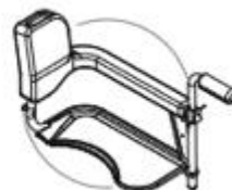
Main frame (integrated with two lift motor columns)
